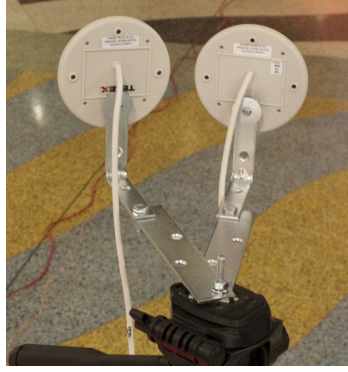
(a) 5dBi directional patch antennas at the prototype full-duplex base station
