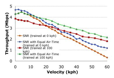
Figure 3.8 Throughput with multipath-induced fading for SNR-based protocols.
