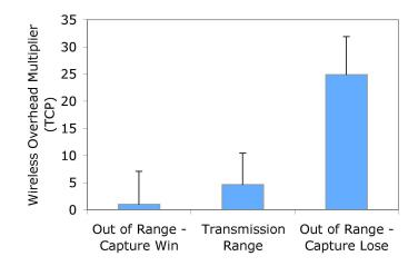
Figure 4.29 WOM considering the different effects of physical layer capture effect within the out of range link class.
