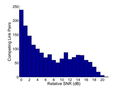
Figure 4.5 Histogram of all competing backhaul link pairs within TFA according to relative SNR.
