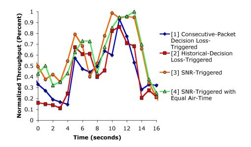
**Figure 3.16** Normalized throughput (from max value in environment) for each of the multirate protocols within a residential urban setting.
