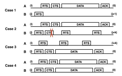
**Figure 4.9** Four cases for symmetric cross-flow connectivity based on timing and capture behaviors.
