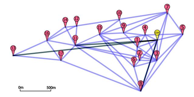
**Figure 2.1** Connectivity graph of the TFA backhaul with appropriate scaling for distance between nodes. There are 4,000 residential users (not shown).
