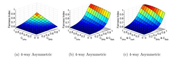
**Figure 4.16** Asymmetric cross-flow connectivity with 2-way handshake (a) and 4-way handshake (b-d) where the disadvantaged flow has increased chance to win the contention due to favorable capture relationships.
