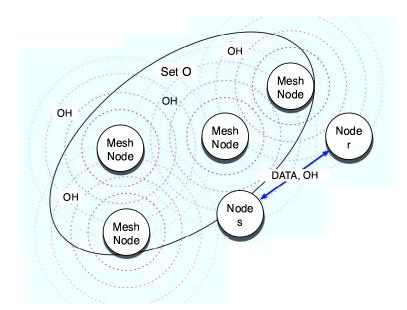
Figure 4.21 Node s sends data and overhead (OH) to node r while all other nodes within set O transmit only OH.
