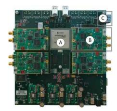
Figure 2.2 WARP FPGA and MIMO-capable radios.
