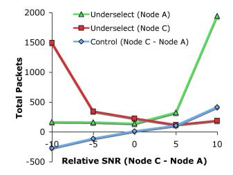
Figure 3.11 Sensitivity to small differences in SNR of competing links with collision/fading differentiation.
