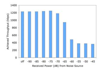
Figure 4.24 802.11 card behavior when noise is injected at the transmitter only. Non-Existence of Carrier Sense Range
