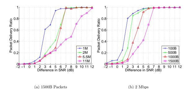
**Figure 4.4** Capture probability of the TFA hardware in-lab on two controlled channels of a channel emulator.
