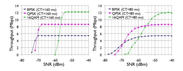
Figure 3.6 Performance of modulation schemes at 0 kph (left) and at 100 kph (right).
