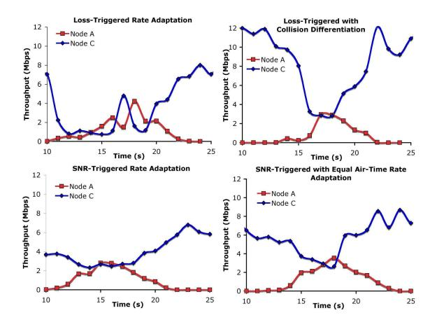
**Figure 3.18** Throughput of each of the four protocols in the heterogeneous links topology (Fig. 3.14).
