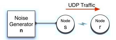
Figure 4.23 802.11-behavior experiment set-up for the off-the-shelf wireless cards.
