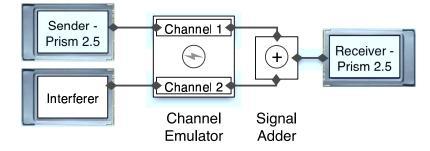
Figure 4.3 Capture experiment set-up for Prism 2.5 Chipset.
