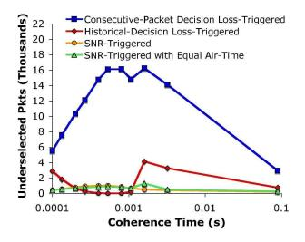
Figure 3.4 Total number of underselected packets per protocol as a function of the coherence time.
