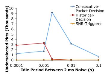
**Figure 3.9** Underselected packets by the loss-triggered protocols as interference is injected.
