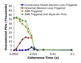
Figure 3.5 Total number of overselected packets per protocol as a function of the coherence time.
