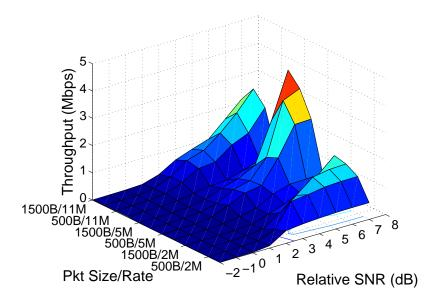
Figure 4.19 Embedded link throughput when hidden source with uncoupled backoff saturates the channel.
