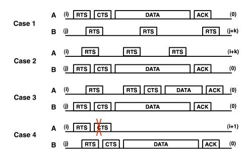
Figure 4.10 Four cases for asymmetric cross-flow connectivity based on timing and capture behaviors.
