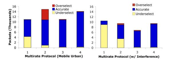
**Figure 3.17** Rate adaptation accuracy with mobile scenario in residential urban setting without (left) and with interference (right).
