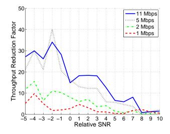
Figure 4.30 Range of throughput reduction multipliers based upon the data rate of the embedded link.
